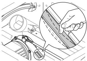
the motor is mounted on a cam plate. The belt tension is adjusted by turning the motor housing as required:
